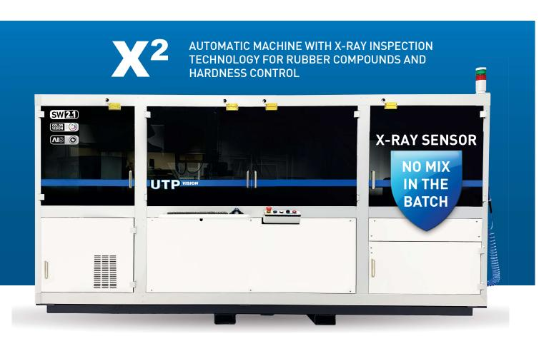
X2 is a revolutionary control system based on X-Ray technology that allows you to check in real time that all the pieces of a production batch are made of the same material. The new sensor allows continuous control without any stop of the pieces and so it guarantees high production rates.
